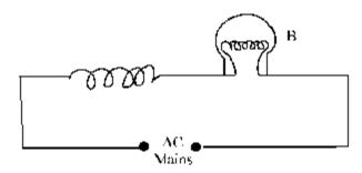
The bulb glows with some brightness. How would the glow of the bulb change if an iron rod were inserted in the coil? Give reasons in support of your answer.
