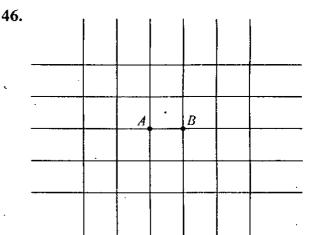
The figure given above shows an infinite wire grid with square cells. The resistance of each wire between neighbouring joint connections is r. What is the resistance of the whole grid between the points A and B?
