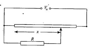
The figure given above shows a potentiometric circuit by means of which one can vary a voltage V applied to a certain device possessing a resistance R. The potentiometer has length l and a resistance  $R_0$  and voltage  $V_0$  is applied to its terminals. What is the voltage fed to the device as a function of distance x?
