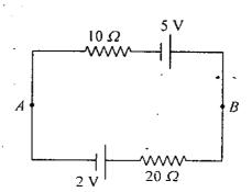
What is the potential difference between the points A and B of the circuit shown above?
