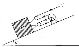
A force F pulls on a mass m using a massless cable and pulley system as shown in the figure given above. What is the acceleration of the block, if the surface is frictionless?
