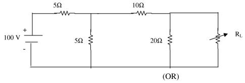
023. For the circuit shown in fig. below, find the current in  $20\Omega$  load resistor, using Thevenin's theorem.
