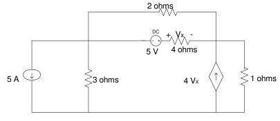
22. Find the current through  $1\Omega$  resistor for the circuit given in Figure using both Thevenin's theorem and Superposition theorem.
