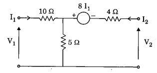
For the network shown in the figure,  $Y_{11}$  and  $Y_{12}$  are, respectively
