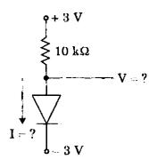
For the circuit shown above, using ideal diode, the values of voltage and current are
