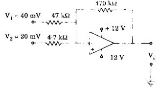
What is the output voltage for the above circuit?
