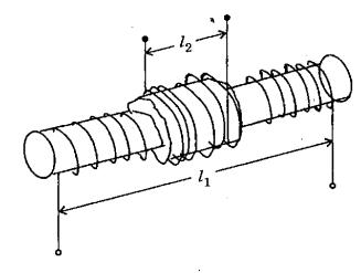
Two coils  $N_1$  and  $N_2$  turns are wound concentrically on a straight cylindrical core of radius r and permeability µ. The windings have length  $l_1$  and  $l_2$  respectively as shown in figure. The mutual inductance will be
