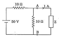
Consider the circuit shown above. The portion of the circuit left to the terminals AB can be replaced by
