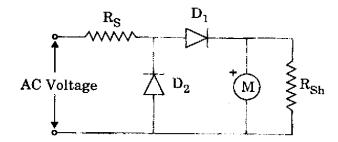
The figure shows the circuit of a rectifier type voltmeter. The diode  ${\rm D}_2$
