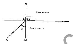
Total Internal Reflection: When a ray of sight travels from denser medium to rarer medium and the angle of incidence becomes greater than the critical angle, then the whote amount of light gets reflected. This is called 'total internal reflection'.
