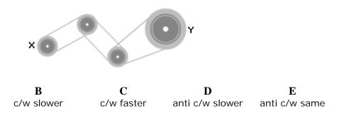
Hint: Where pulley wheels are driven by belts, they rotate in the same direction. Smaller wheels will turn faster that larger wheels.
