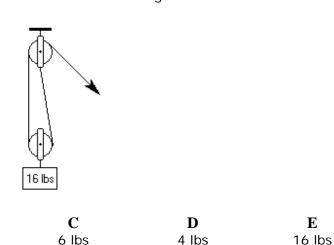
Hint: If the pulley is fixed, then the force required is equal to the weight. If the pulley moves with the weight then the force is equal to half of the weight. Another way of thinking about this is to divide the weight by the number of sections of rope supporting it to obtain the force needed to lift it.
