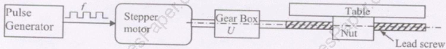
Q.84 The Basic Length Unit (BLU), i.e., the table movement corresponding to 1 pulse of the pulse generator, is
