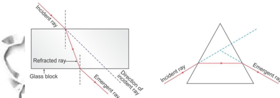
When a light ray passes through a prism, it bends towards the base of the prism. Hence, incident ray and emergent ray are not parallel to each other as they are in case of a glass slab.
