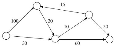
(b) Determine the critical path for the following Project Network:
