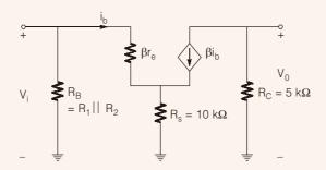
$$\begin{split} &V_i = \beta i_b r_e + (i_b + \beta i_b) \ R_s \\ &V_i = \beta i_b r_e + i_b (1 + \beta) \ R_s \\ &V_i = i_b [\beta r_e + (1 + \beta) \ R_s] \\ \end{split} \qquad ...(i) \end{split}$$
