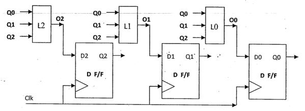
The minimized expressions for O0, O1 & O2 are : a.  $O_2 = Q_2$   $O_1 = Q_1$   $O_0 = Q_0$
