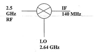
a. IF Spectrum is inverted and image is at 2.780 GHz
