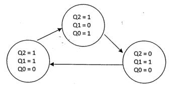
It is designed using D F/Fs and combinational logic blocks  $L_1$ ,  $L_2$  &  $L_3$  and is initialized at ( $Q_2$ =1,  $Q_1$  = 0,  $Q_0$  = 1)
