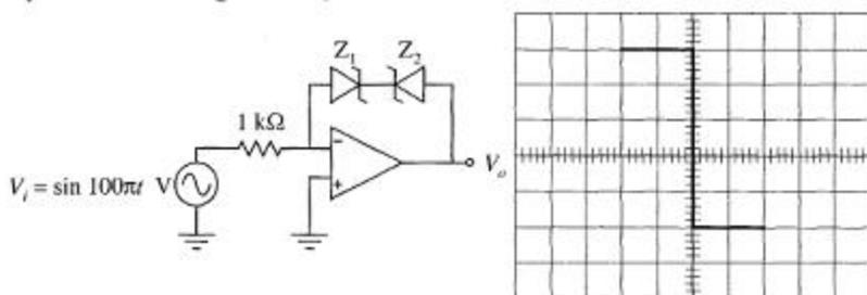
Assuming that the opamp is ideal and the zener diodes have forward biased voltage drop of  $0.7\text{ V}$ , the values of reverse break-down voltages of  $Z_1$  and  $Z_2$  are, respectively.
