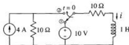
The current  $i$  through the inductor for  $t \geq 0$  is
