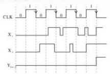
This is a synchronous circuit, so both the flip flops will trigger at the same time and will respond on falling edge of the Clock. So, the correct output (Y) waveform is associated to w<sub>3</sub> waveform.
