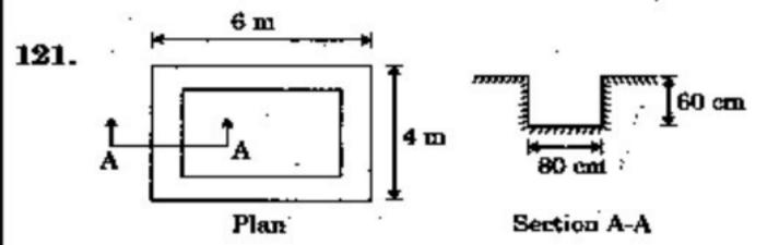
The above figure represents plan and section of an excavation layout. The volume of earthwork in excavation of foundation trench is
