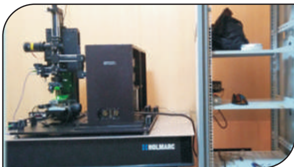
Working prototype of Microfluidic-based, Laser-assisted Bovine Sperm Sorting (MLBSS) System developed by Jiva Sciences Pvt. Ltd., Bengaluru
