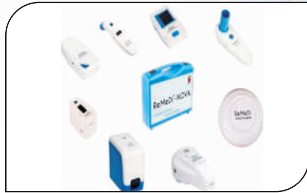
ReMeDi NOVA – A device consisting of multiple sensors with a common access interface, that can be used to provide a wide range of diagnostics at the point of care has been developed by Neurosynaptic, Bengaluru
