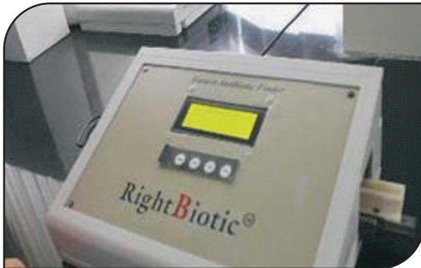
A point-of-care (POC) device for testing antibiotic sensitivity of different bacteria found in human urine that are responsible for Urinary Tract Infection (UTI). Developed by Xcellence in Bio Innovations, Bits-Pilani, Hyderabad
