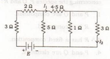
In this circuit the ratio of currents  $I_1/I_2$  is
