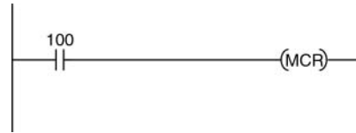
Figure 1.8 Master Control Relay
