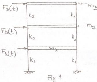
Take storey height 'h', modulus of elasticity 'E' and moment of inertia as 'I'.
