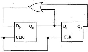
For the circuit shown, the counter state  $(Q_1Q_0)$  follows the sequence:
