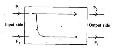
For the above directional coupler a coupling factor in dB is:
