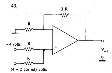
The output of the above OP-amp circuit is:
