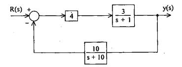
The characteristic equation of the above closed-loop system is:
