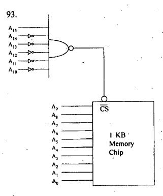
Consider a memory chip with 1024 bytes storage connected to a 8085 chip address lines (or any microprocessor with 16 address lines) as above. What is the range of memory address?
