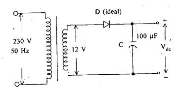
The output  $V_{dc}$  from the above circuit is:
