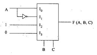
A  $4\times1$  MUX is used to implement a 3-input Boolean function is as shown above. The Boolean function F(A, B, C) implemented is:
