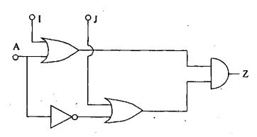
The circuit shown above is to be used to implement the function  $Z = f(A, B) = \overline{A} + B$ . The values of I and J are:
