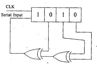
The shift register shown in the given figure is initially loaded with the bit pattern 1010. Subsequently the shift register is clocked, and with each clock pulse the pattern gets shifted by one bit position to the right. With each shift, the bit at the serial input is pushed to the msb position. After how many clock pulses will the content of the shift register become 1010 again?
