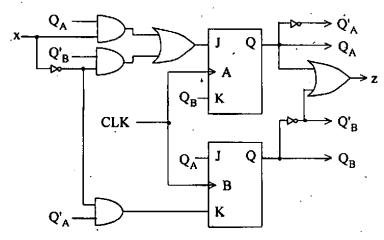
Analyze the sequential circuit shown above in figure. Assuming that initial state is 00, determine what input sequence would lead to state 11?
