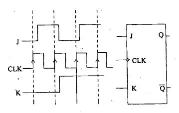
The J-K flip-flop shown above is initially reset, so that Q = 0. If a sequence of four clock pulses is then applied, with the J and K inputs as given in the figure, the resulting sequence of values that appear at the output Q starting with its initial state, is given by:
