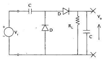
Consider the above circuit, for  $V_i = V_m \sin \omega t$ , the output voltage  $V_o$  for  $R_L \to \infty$  will be:
