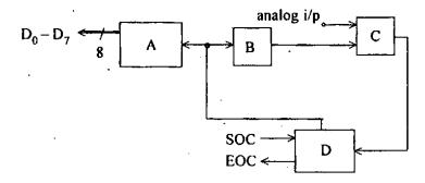
Consider the above block diagram of a successive approximation A/D converter. Match List-I with List-II and select the correct answer using the code given below the lists:
