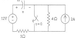
b) Calculate i(t) for t > 0 in the circuit given below using Laplace transform method.
