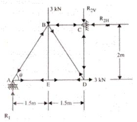
b. Fig.2 shows a truss ABCDE, hinged at C and roller supported at A. At the point B, a vertical force of 3 kN and at D, a horizontal force of 3 kN are applied. Determine the reactions at supports and forces in the members of the truss. (12)
