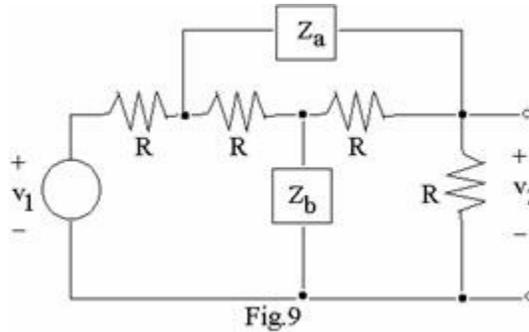
b. Synthesize  $Z_a$  and  $Z_b$  if  $\frac{V_2}{V_1} = \frac{2s^2 + 1}{s^3 + 4s^2 + 5s + 2}$  and  $R = 1$ . (6)
