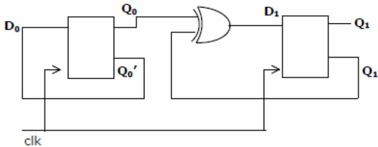
The flip-flops are positive edge triggered D FFs. Each state is designated as a two-bit string  $Q_0 Q_1$ . Let the initial state be 00. the state transition sequence is
