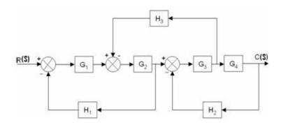
b. Develop the signal flow graph and determine the overall transfer function of the given system using Mason's Gain formula (8)
