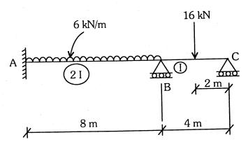
Moment of inertia of the beams is shown in the circles.
