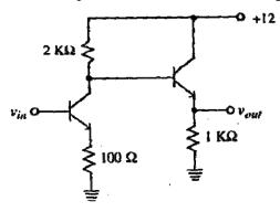
If  $v_{in}$  is +1 V, what is the value of  $v_{out}$ ? If  $v_{in}$  is changed to +3 V, what is the value of  $v_{out}$ ? What is the output voltage compliance (maximum voltage range that the output can swing when the input is varied) of the circuit?
