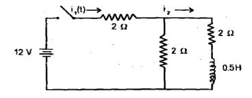
(b) The switch S is kept open until steady state is reached by the network shown below. At t = 0, S is closed
