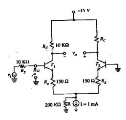
The transistors have  $\beta=100$ . Determine input differential resistance  $R_{id}$ , overall voltage gain  $v_0/v_i$  and the worst case common mode rejection ratio if the two collector resistances are accurate to within  $\pm 1\%$ .
