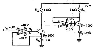
If the load resistance is 500  $\Omega$  what is the load voltage? If the load resistance is reduced to zero what is the load current?
