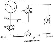
Which of the following connections, and the corresponding phase shift  $\theta$ , should be used for the transformer between A and B?
