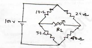
b) Determine the output voltage  $V_{\rm out}$  in the circuit shown.
