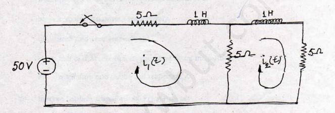
b) Find the The venin's equivalent for the circuit shown in the figure below:
