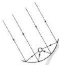
Figure 5a: Focusing solar radiation with a parabolic mirror
