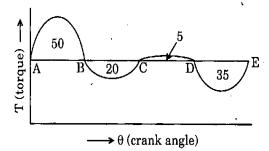
The crank-effort diagram of an engine running a machine is showing the areas above and below the mean line (in joules). What is the maximum fluctuation of energy in the above diagram?
