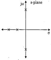
The roots of the characteristic equation of a linear control system are shown in the figure as above with cross (x) marks. What can be said of the system?
