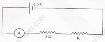
When the circuit is switched on, the ammeter reads 0.5 A.
