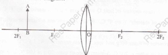
Copy the diagram and using three rays starting from point A, obtain the image of the object formed by the lens.
