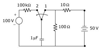
In the above circuit, the switch has been in position 1 for quite a long time. At t = 0 the switch is moved to position 2. At this position what is the time constant?
