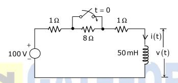
In the above circuit, the switch is open for a long time. At time t = 0, the switch is closed. What are the initial and final values of voltages across the inductor?
