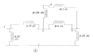
15. For the system network shown in figure, find the sub transient current from generator 1, line (1), (2) and the bus voltages (1) and (3) for a 3 phase fault at bus.(2)
