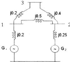
Assume that no current is flowing prior to the fault and that the pre fault voltage at bus (2) is  $1.0\angle0$  p.u. Use the bus impedance matrix for calculations.
