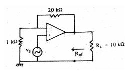
An Op-amp with an open-loop gain of 10,000.  $R_m = 2 \ k\Omega$  and  $R_O = 5000$  is used in the non-inverting configuration as shown in the above figure. The output resistance  $R_{of}$  is
