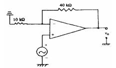
The Op-amp in the above circuit shows a unity-gain bandwidth of 1 MHz and a dominant pole at 10 Hz. The bandwidth of the non-inverting amplifier will be
