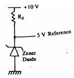
A 5 V reference is drawn from the circuit shown in the above figure. If the zener diode is of 5 mV and 5 V, then  $R_Z$  will be
