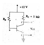
Assume  $V_{BE} = 0.7$  V and  $\beta = 50$  for the transistor in the circuit shown in the above figure. For  $V_{CE} = 2$  V, the value of  $R_B$  is
