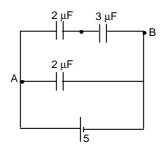
Charge across the combination of 2  $\mu$ F and 3  $\mu F$  = charge across 3  $\mu F$
