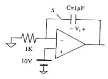
In the figure shown above, the OP AMP is supplied with  $\pm$  15V and the ground has been shown by the symbol  $\nabla$ .
