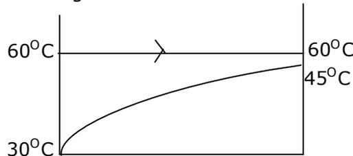
$$\Delta T_1 = 30^\circ\text{C}, \Delta T_2 = 15^\circ\text{C}, \text{LMTD} = \frac{\Delta T_1 - \Delta T_2}{\ln\left(\frac{\Delta T_1}{\Delta T_2}\right)} = \frac{30 - 15}{\ln\left(\frac{30}{15}\right)} = 21.6^\circ\text{C}$$
