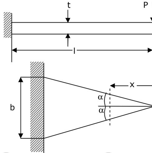
52. The area moment of inertia about the neutral axis of a cross-section at a distance  $x$  measured from the free end is
