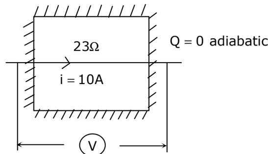
$$W_{\text{electric}} = i^2 R = (10^2 \times 20) \text{ watts} = -2.3 \text{ kw (on system)}$$
