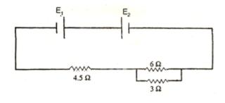
Calculate the value of current flowing through the resistance of  $\frac{3\Omega}{2}$
