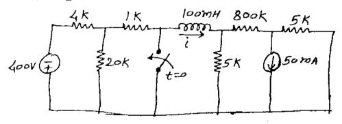
Using superposition theorem, find  $V_{\rm x}$  —
