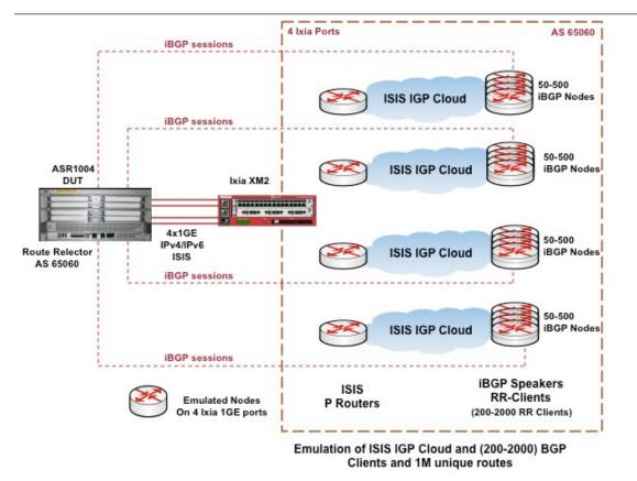
Figure 2: Cisco ASR1004 RP2 Route-Reflector Convergence and Scaling Test Setup
