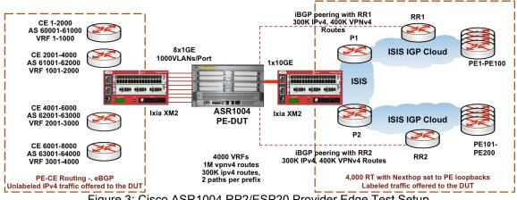
Figure 3: Cisco ASR1004 RP2/ESP20 Provider Edge Test Setup
