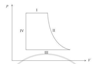
Which of the labelled parts of the cycle identify isobaric changes and adiabatic changes of state?
