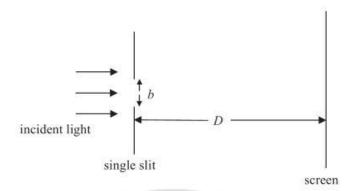
Which of the following changes, carried out separately, in respect of b and D will result in an increase in width of the first diffraction maximum formed on the screen?
