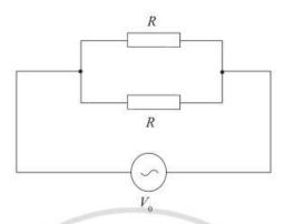
The resistance of each resistor is R and the peak voltage of the ac supply is  $V_{\theta}$ . Which of the following is the average power dissipated in the circuit?
