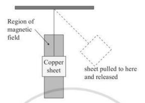
The uniform magnetic field is directed into the plane of the paper.
