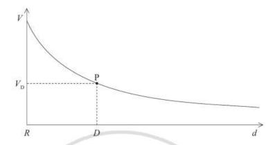
The magnitude of the electric field strength at a point P a distance D from the centre may be defined as
