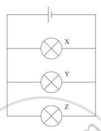
The cell has negligible internal resistance. The filament of lamp Y breaks such that its resistance becomes infinite.
