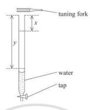
The tap at the base of the tube is opened. As the water runs out, the sound is loudest when the water level is a distance x below the top of the tube. A second loud sound is heard when the water level is a distance y below the top. Which **one** of the following is a correct expression for the wavelength  $\lambda$  of the sound produced by the tuning fork?
