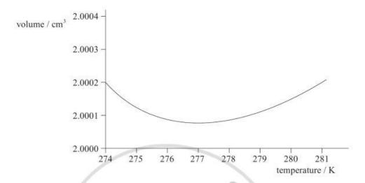
A thermometer is to be designed that measures temperatures in the range between 274 K and 280 K.
