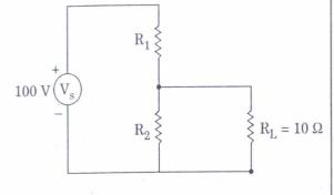
What is the voltage across the load resistance,  ${\rm R}_{\rm L}$  in the above circuit ? The value of each resistor connected in the circuit is  $10 \Omega$ .
