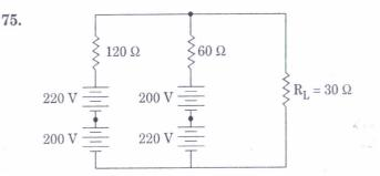
In the circuit shown above, the current through R<sub>L</sub> is
