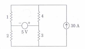
The power dissipated in the 1  $\Omega$  resistor is 1 W due to the 5 V voltage source alone and 576 W due to 30 A current source alone. The total power absorbed in the same resistor due to both the sources is
