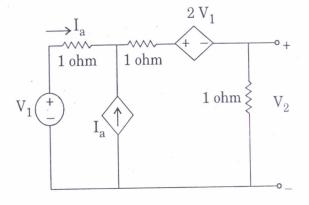
The above network contains resistors and controlled sources.  $G_{12} = \frac{V_2}{V_1}$  is
