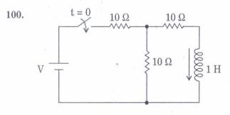
The value of V that would result in a steady-state current of 1 A through the inductor in the above circuit is
