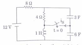
In the circuit shown above, the switch is closed after a long time. The current  $i_{S}(0^{+})$  through the switch is
