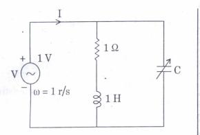
In the above circuit, the value of C for the circuit to exhibit a power factor of 0.86, is approximately
