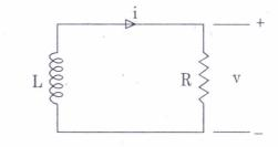
Voltage and current expressions for the above circuit are given at  $t \ge 0$  as  $v = 125 e^{-50t} V$ ,  $i = 5 e^{-50t} A$ . The value of L will be
