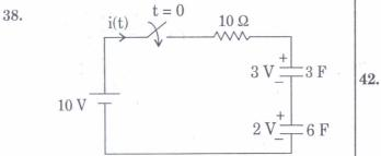
In the circuit shown above, switch S is closed at t = 0. The time constant of the circuit and initial value of current i(t) are
