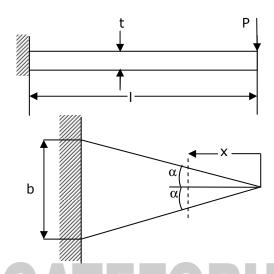
52. The area moment of inertia about the neutral axis of a cross-section at a distance x measured from the free end is  $\frac{bxt^3}{6l}$  (B)  $\frac{bxt^3}{12l}$  (C)  $\frac{bxt^3}{24l}$  (D)  $\frac{xt^3}{12}$
