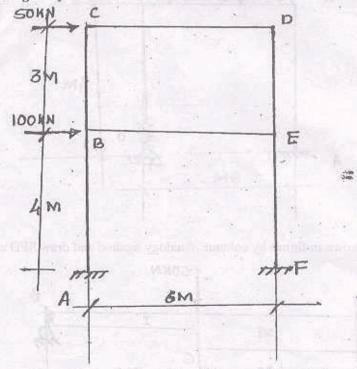
Analyse the pin-jointed frame shown in figure by stiffness matrix method and calculate member forces and member displacements.
