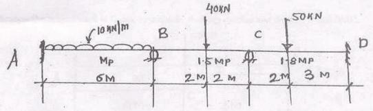
(a) For the beam shown in figure construct ILD for (i) V<sub>B</sub> (ii) BM at C. Show the ordinates at 2 M intervals.
