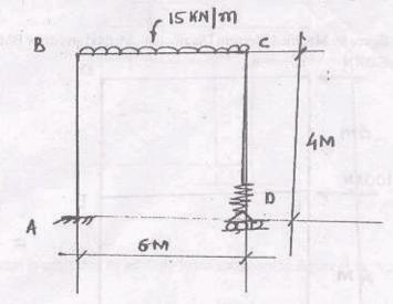
(a) Analyse the beam shown in figure by column. Analogy method and draw SFD and BMD.
