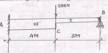
(b) For the non prismatic beam element shown in figure. Calculate the stiffness co-efficients K<sub>11</sub> and K<sub>21</sub>. Also calculate C.O.F. from B to A.
