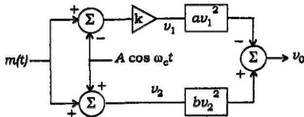
What would be the value of gain  $k$  in figure above to yield the suppressed carrier DSB signal?
