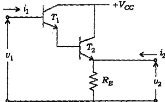
For the Darlington amplifier shown in figure above, obtain its Z-matrix for identical  $T_1$  and  $T_2$  having  $h_{fe} = 100$ ,  $R_E = h_{ie} = 1 \text{ k}$
