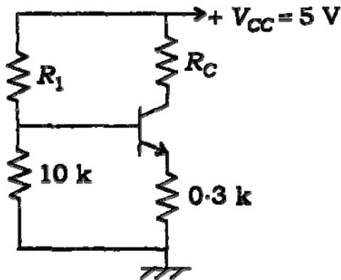
The BJT in amplifier of figure above has  $h_{fe} = 100$ ,  $V_{BE} = 0.7V$ ,  $I_{CO} = 0$ . Calculate the values of  $R_1$  and  $R_C$  such that its  $I_C = 1 \text{ mA}$  and  $V_{CE} = 2.5 \text{ V}$ .
