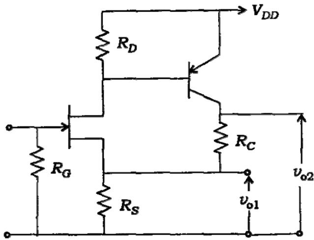
Obtain  $v_{o1}$  and  $v_{o2}$  in figure above.
