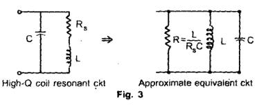
For a practical tank circuit shown in Fig. 4 below, the resonance occurs a 1 MHz. Assuming a high Q-coil, find out the quality factor of high-Q coil at resonance frequency.
